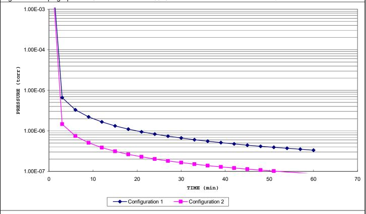
These vacuum performance projections are not a guarantee of system performance. This model accounts for residual air removal and approximates water outgassing from metal surfaces and o-ring permeation; the model does not account for real or virtual leaks or poor assembly techniques (e.g. poor cleanliness). These results are not to be used as performance specifications.
