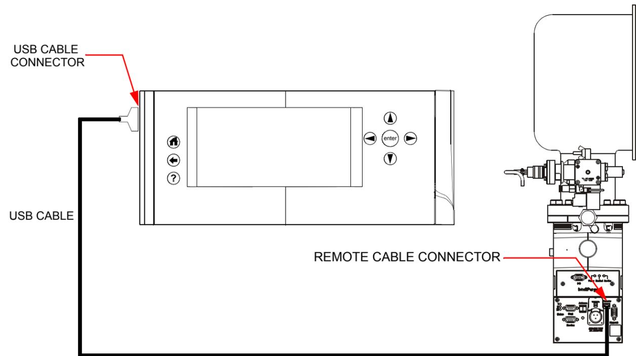
Figure 3: On-Board *IS* Remote Cable Connections to an On-Board *IS* Cryopump
