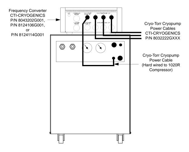
Figure 3-11: 1020R Compressor with Cryo-Torr Cryopumps
