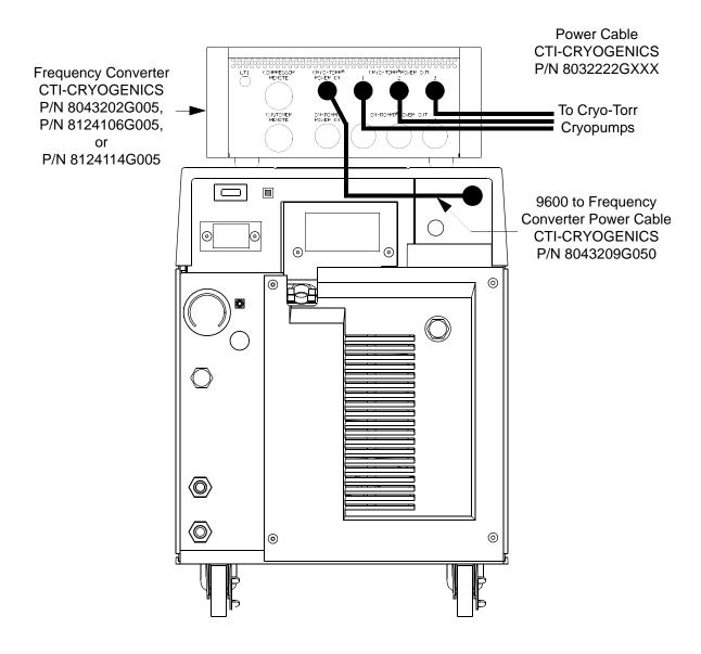
Figure 3-2: 9600 LV Compressor with an Cryo-Torr Cryopumps
