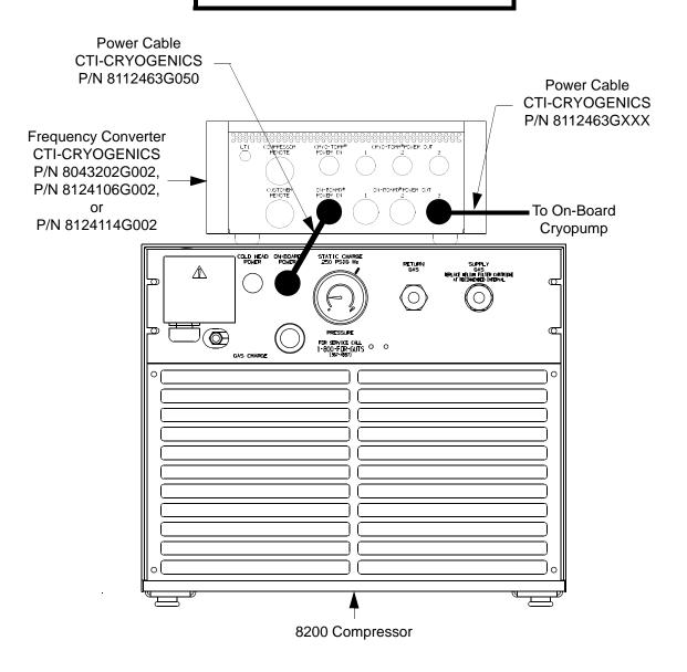
Figure 3-5: 8200 Three-Phase Compressor with an On-Board Cryopump
