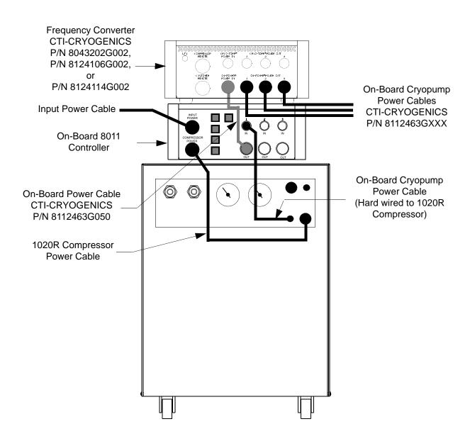
Figure 3-10: 1020R Compressor with On-Board Cryopumps
