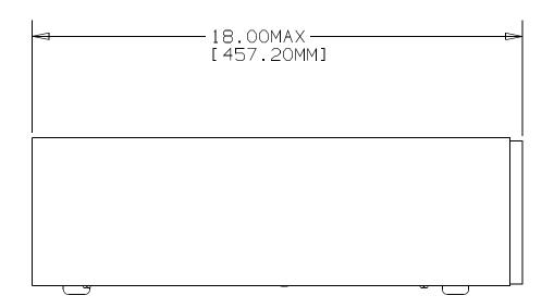
Figure 1-2: Frequency Converter Dimensions
