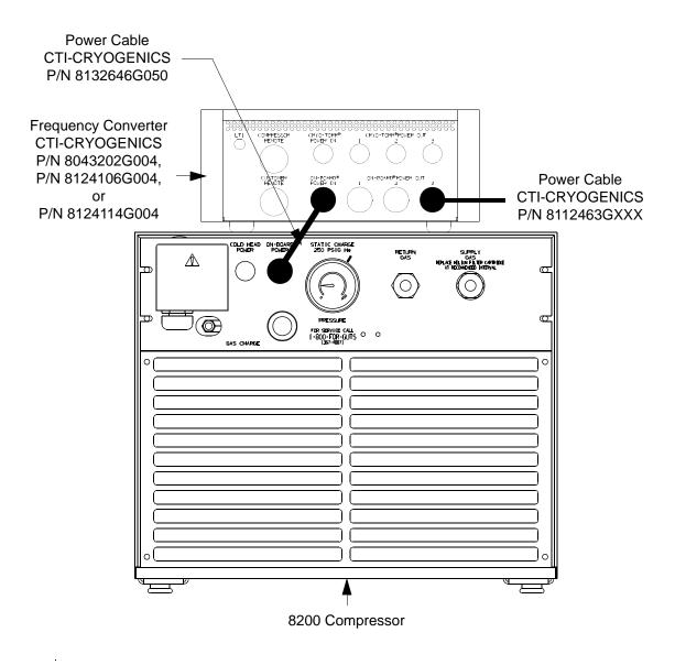
Figure 3-3: 8200 Single Phase Compressor with an On-Board Cryopump
