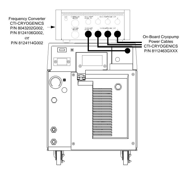
Figure 3-1: 9600 LV Compressor with On-Board Cryopumps
