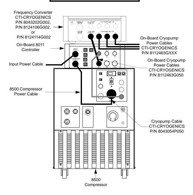
Figure 3-8: 8500 Compressor with an On-Board Cryopump
