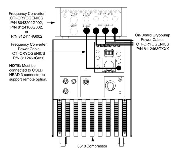
Figure 3-7: 8510 Compressor with On-Board Cryopumps
