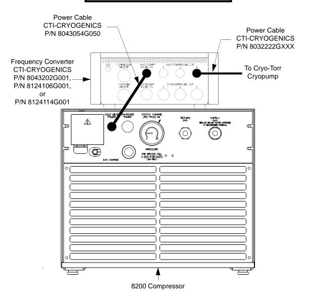
Figure 3-6: 8200 Three-Phase Compressor with Cryo-Torr Cryopumps
