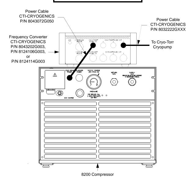
Figure 3-4: 8200 for Single Phase Compressor with Cryo-Torr Cryopumps
