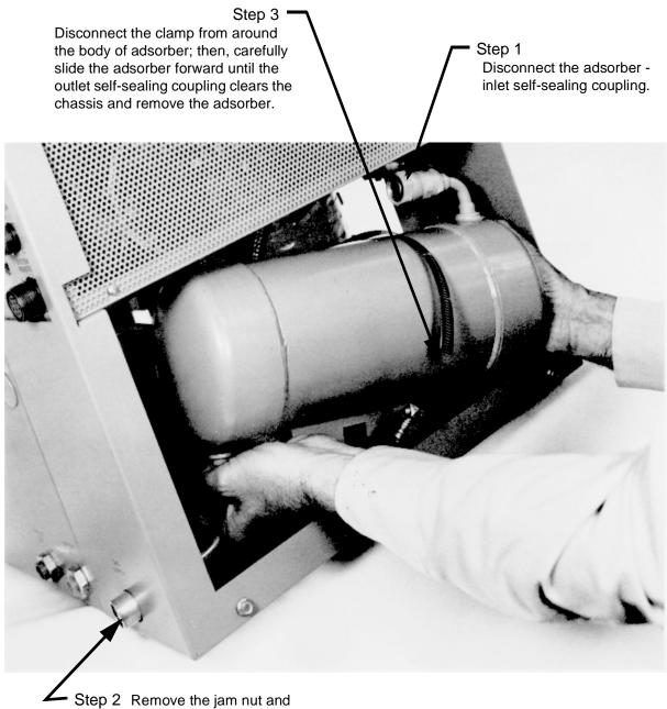
2 Remove the jam nut and washer that secure the adsorber-outlet self-sealing coupling to its chassis.
