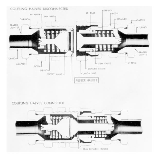
Figure 4: Cutaway Views of a Self-Sealing Coupling (Aeroquip)
