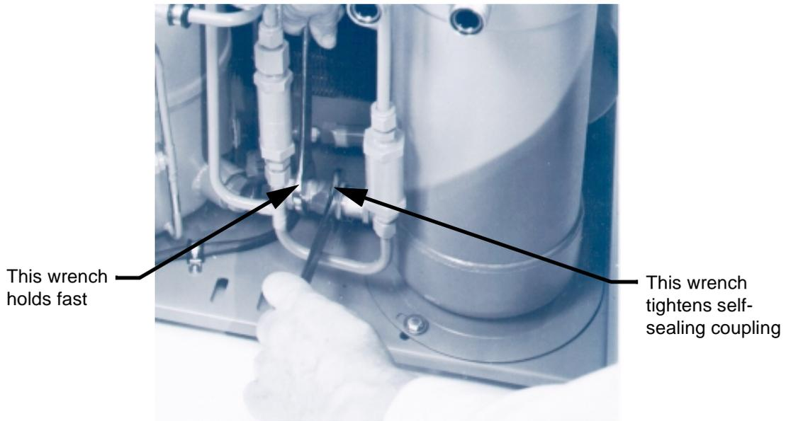
**Figure 3: Proper Method for Connecting Self-Sealing Couplings**
