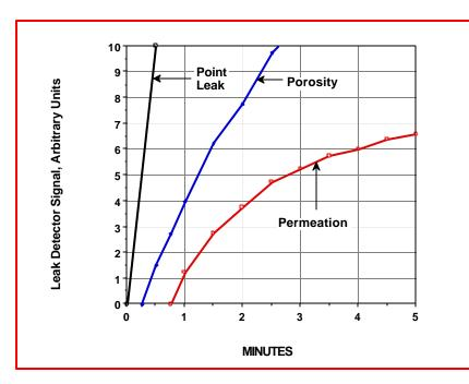
Permeation is differentiated from real leaks by the fact that the rates are not controlled by the molecular weight of the gas as is found with real leaks. There is a much more complex mechanism at work. If we form a mental picture of the internal diffusion pathway through an O-ring as a capillary tube that's hundreds of meters long and crumpled into a ball, we can easily see that the permeating
