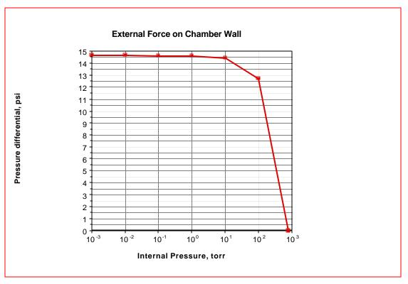
As the pressure within the vacuum chamber is reduced, the ambient pressure increases the force on the chamber wall, but the increase in force is negligible below a few torr.
