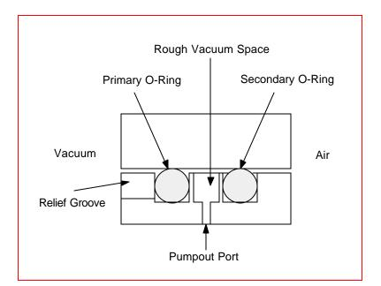
The relief groove allows trapped volumes of gas to be pumped out of the O-ring groove and the rough vacuum space with pumpout reduces the primary O-ring's permeation rate. Source: Phil Danielson
