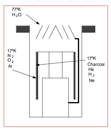
The various cold arrays within the cryopump body show their specific pumping capability. The chevrons in the pump inlet are positioned to pump the main gas load in most systems, water vapor. Other gases pass though the water pumping array, and are then pumped according to their degree of possible condensation.
