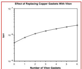
compromise. If, for example, a flange is to be installed and left in place for long periods, the extra trouble of using copper with its requirement of a lot of bolts, high bolt torque, and installation time is negligible. If, though, a flange is to be opened and closed frequently, the ease and speed of using an elastomer gasket is often a good trade-off against the higher permeation rate.
