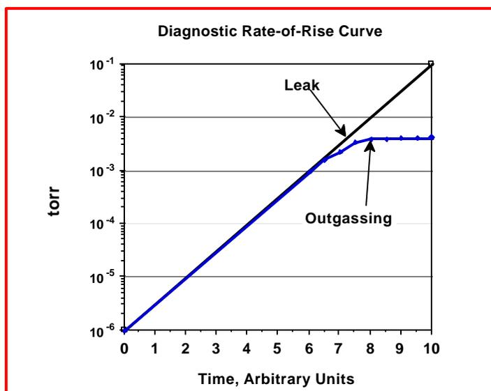
A standard rate-of-rise curve should be established, as with a pumpdown curve, for any system when it is performing properly. The best way of handling them together will depend upon their type of system control and instrumentation provided. A manually operated system can have the operator compare the pumpdown and rate-of-rise readings with a graph
