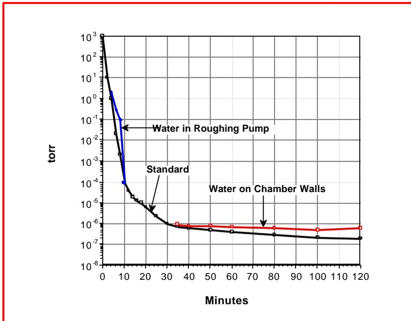
*Comparing a pumpdown curve to a standard curve can be used to detect problems such as water vapor condensing in a roughing pump or a build-up of water vapor on chamber surfaces.*
